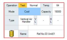
Detail tab- After approximately (30) to (40) minutes of run time, use the "Check List" feature to confirm operating variables are within range.
